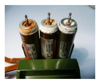
Original Motors survived 100 cycles autoclaving – but 5 min. in saltwater
